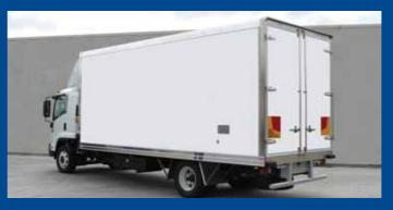
rigid body and offer far greater thermal insulation than aluminium or steel wall reinforcements.
